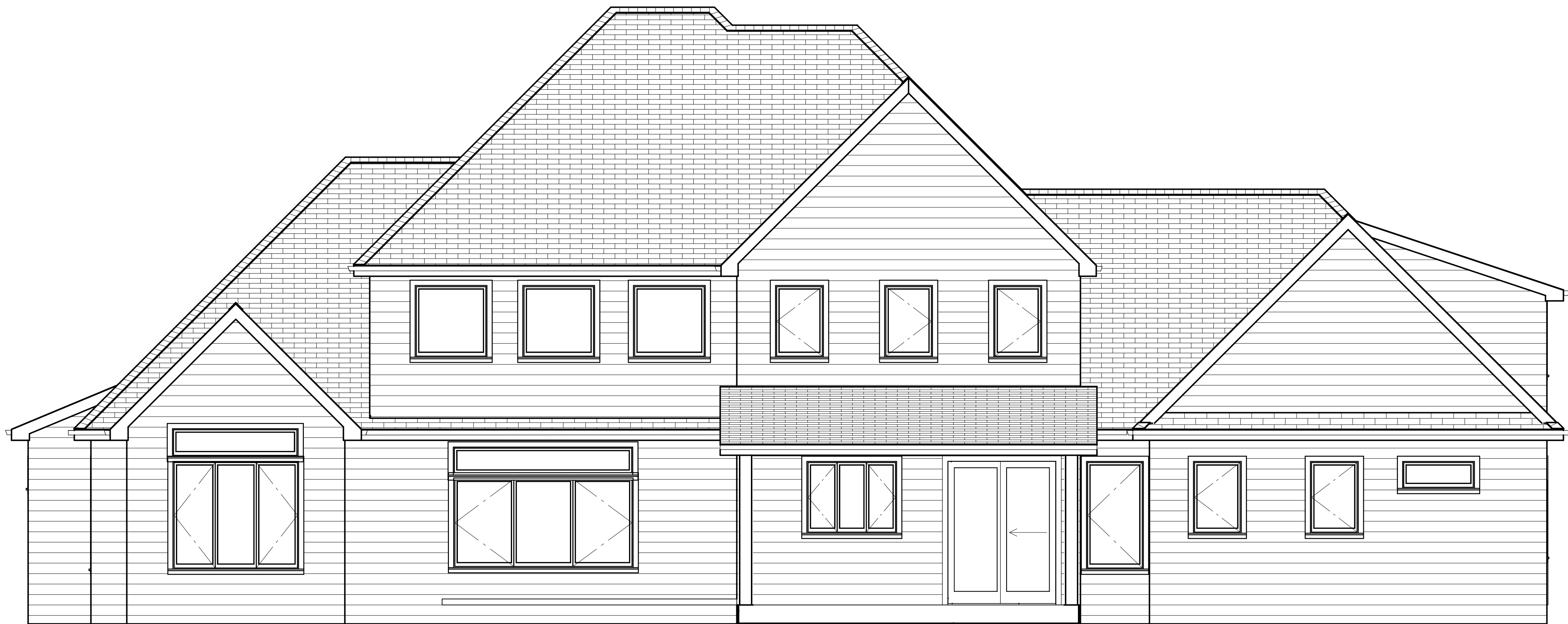
E3 EXTERIOR ELEVATION BACK 1/4 IN = 1 FT
