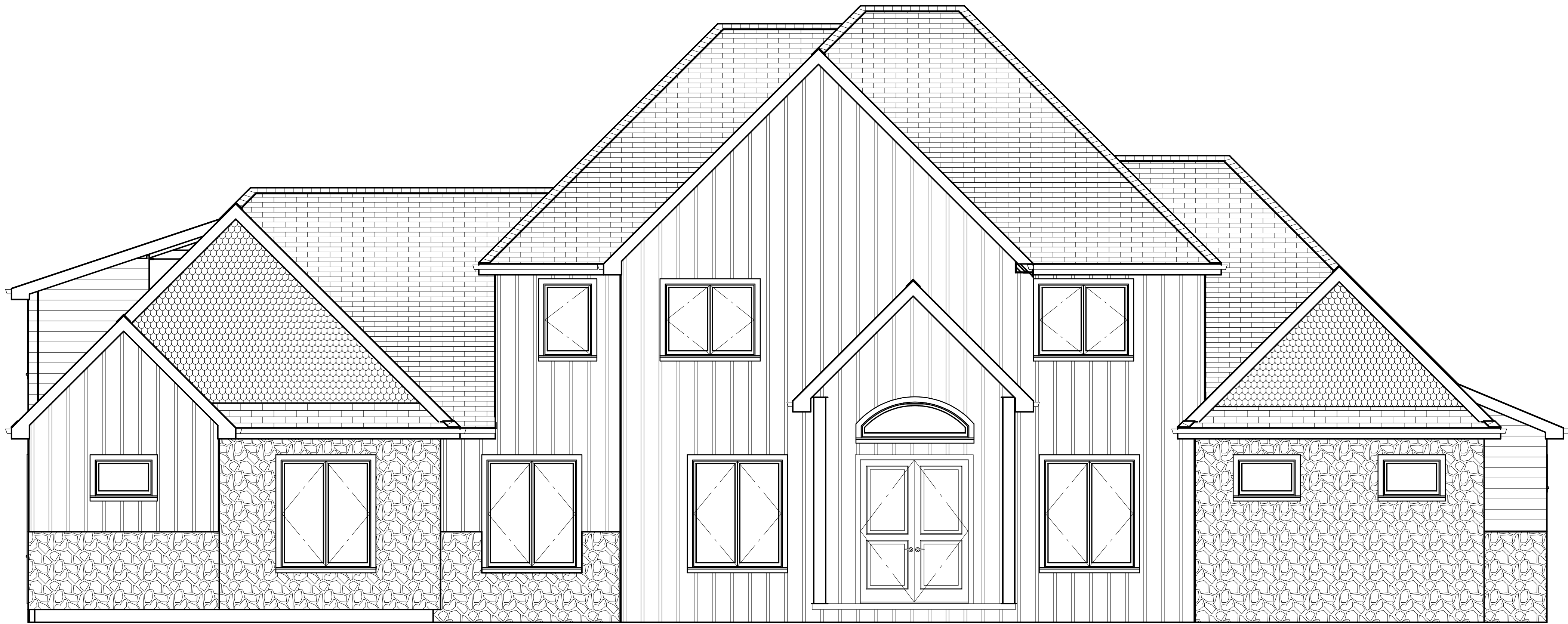
E1 EXTERIOR ELEVATION FRONT 1/4 IN = 1 FT
