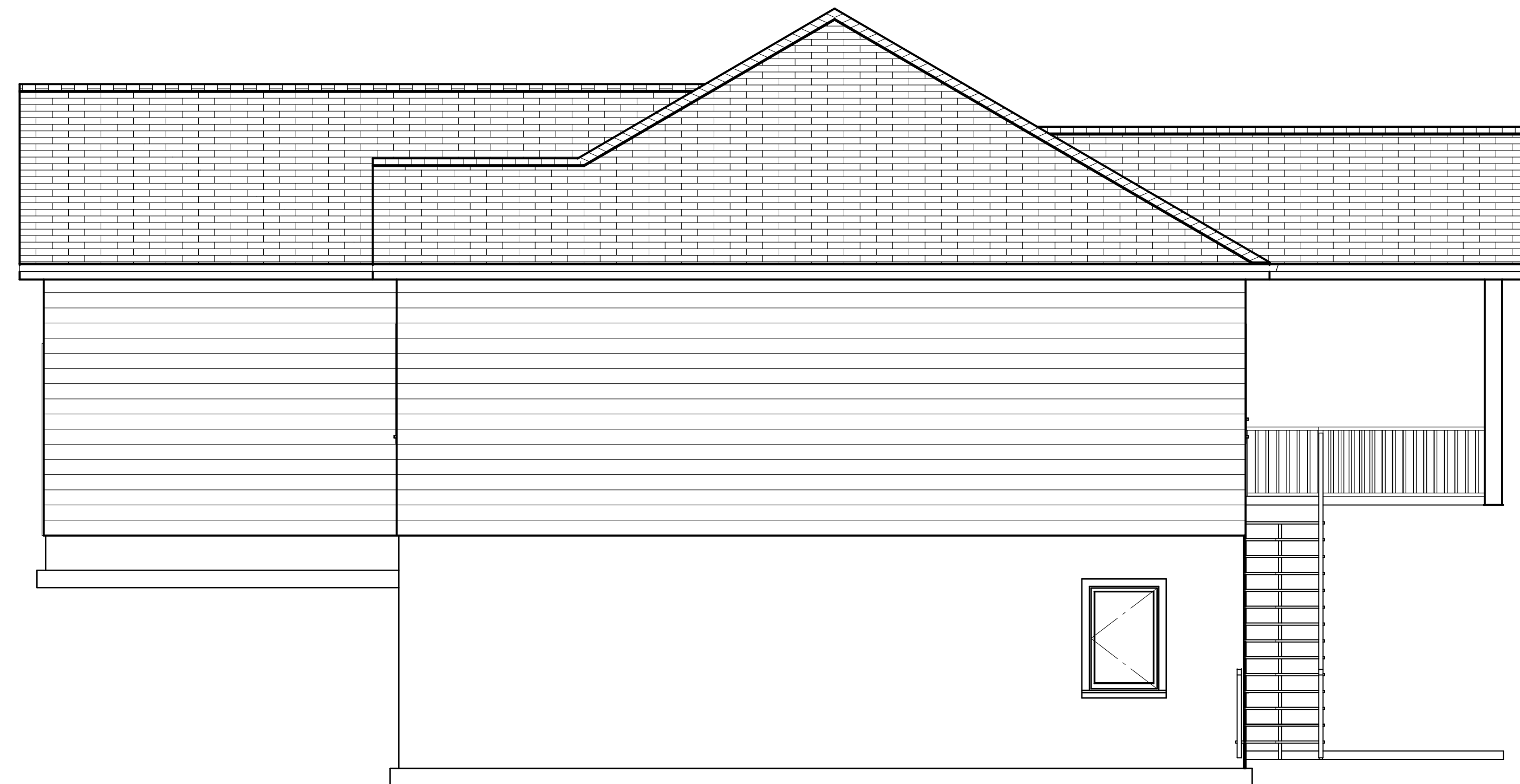
E4 EXTERIOR ELEVATION RIGHT 1/4 IN = 1 FT
