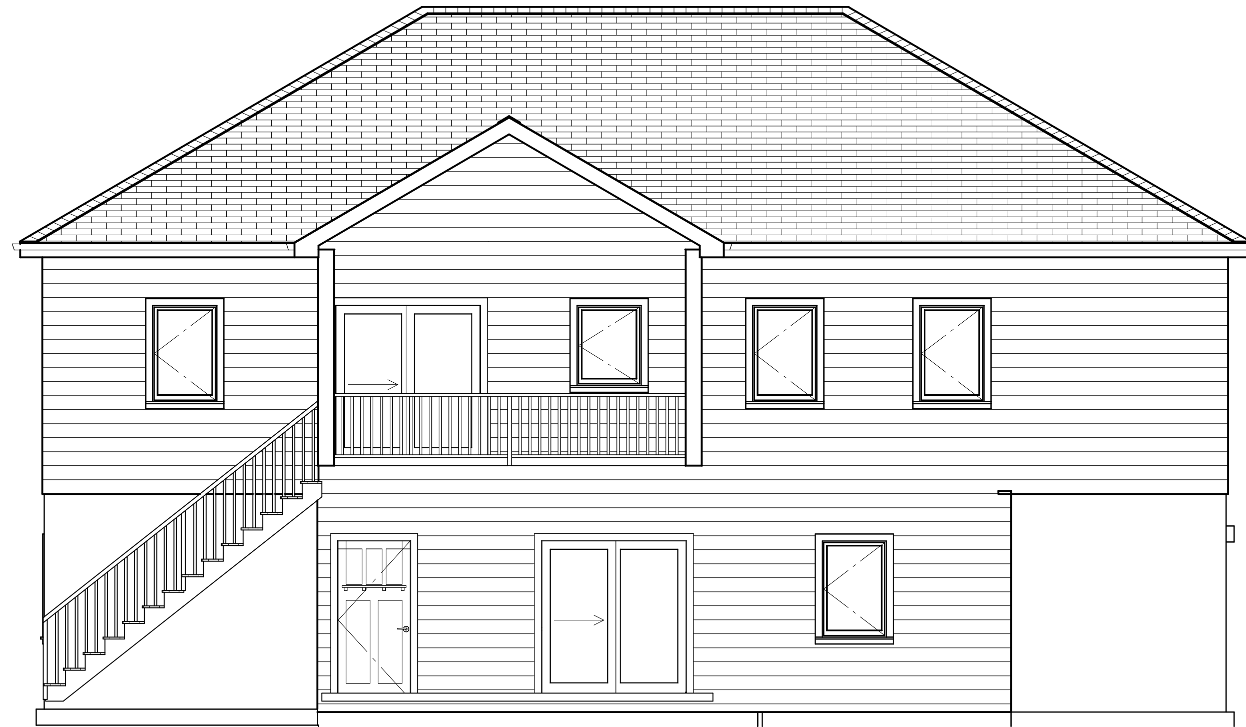
E3 EXTERIOR ELEVATION BACK 1/4 IN = 1 FT
